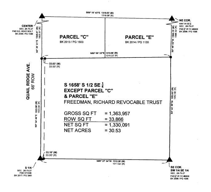
Basis of Bearing is Iowa State Plane Coordinate System South Zone.
