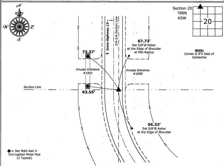
Northeast Corner of the NW 1/4-NW 1/4 of Section 20-89-5 Set 1"Ø Bronze Survey Marker PLS 19211
