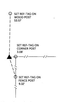
**CENTER OF SECTION** SET 1/2" REBAR W/ORANGE CAP #17939
