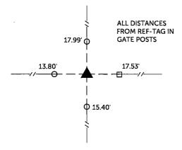
NW CORNER NE 1/4 - NW 1/4 SET 1/2" REBAR W/ORANGE CAP #17939
