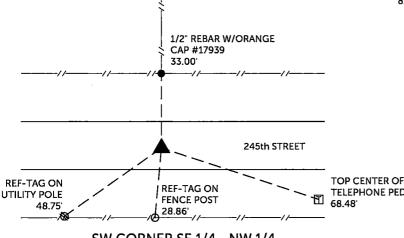
SW CORNER SE 1/4 - NW 1/4 SET 1/2" REBAR W/ORANGE CAP #17939
