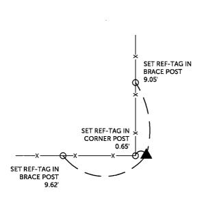
NE CORNER SW 1/4 - NW 1/4 SET 1/2" REBAR W/ORANGE CAP #17939
