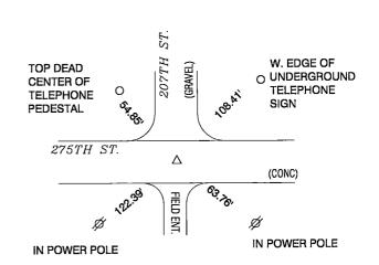
LEGEND: (MONUMENT SYMBOLS ARE ORIENTED TO THE NORTH) PLSS CORNER (as noted) S ▲ 5 • RECORD TIE (as noted) PLSS CORNER - 1/2" DIAMETER x 30" IRON REBAR w/ORANGE PLASTIC ID CAP (#17162) SET 0 TAG (as noted) List Corners to be Indexed
