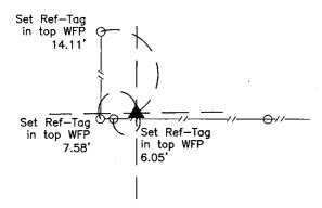
SW Cor. SE 1/4-NE 1/4 Set 1/2"Ø Rebar w/Orange Plastic Cap PLS 17939
