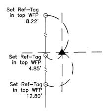
NW Cor. SE 1/4-NE 1/4 Set 1/2"Ø Rebar w/Orange Plastic Cap PLS 17939
