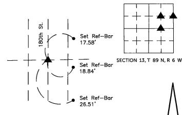
NE Cor. SE 1/4-NE 1/4 Set 1/2"Ø Rebar w/Orange Plastic Cap PLS 17939
