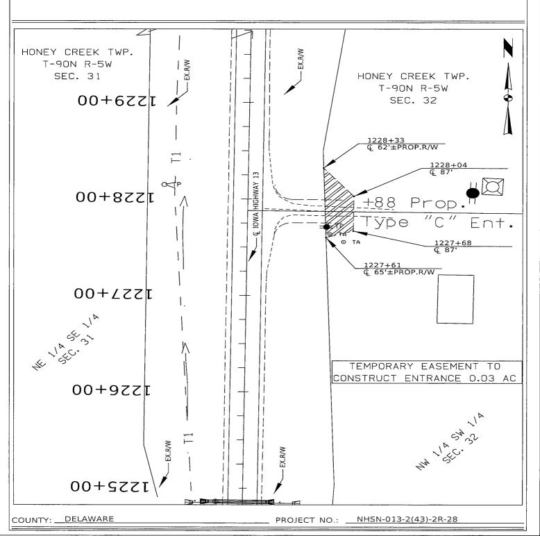
IOWA DEPARTMENT OF TRANSPORTATION RIGHT OF WAY BUREAU PLOT PLAN PARCEL NO.: 34 OWNER: Estate of Arlene T Jones SECTION: 31 T 90 N-R 5 W. LEGEND W.D. OR EASEMENT LINE: SCALE:1"=\_\_\_\_50' ACCESS LOCATION POINT: PROPERTY LINE: 1235+00 +17 Exist. Type "C" Ent. +00 Prop. Type "C" Ent. 00+787 1233+00 TEMPORARY EASEMENT TO CONSTRUCT ENTRANCE 0.01 AC HONEY CREEK TWP. HONEY CREEK TWP. T-90N R-5W T-90N R-5W SEC. 31 SEC. 32 1737+00 1231+00
