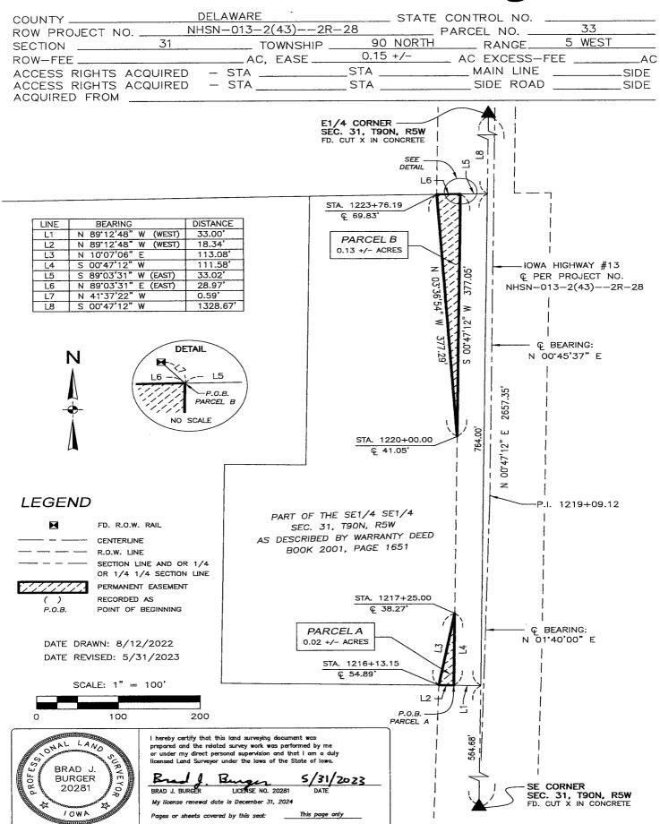
IOWA DEPARTMENT OF TRANSPORTATION RIGHT OF WAY BUREAU PLOT PLAN PARCEL NO.: 33 OWNER: Joseph W & Becky L Kafer SECTION: 31 T 90 N-R 5 W. LEGEND SCALE:1"=\_\_\_\_50' W.D. OR EASEMENT LINE: ACCESS LOCATION POINT: 1220+00 TEMPOARARY EASEMENT TO CONSTRUCT ENTRANCE & SHAPE 0.06 AC 1518+00 1218+41 Q 67' +25 Prop. Type "C."--1217+00 1216+92 **Q** 43'±PROP.R/W HONEY CREEK TWP HONEY CREEK TWP. T-90N R-5W T-90N R-5W SEC. 32 SEC. 31 0
