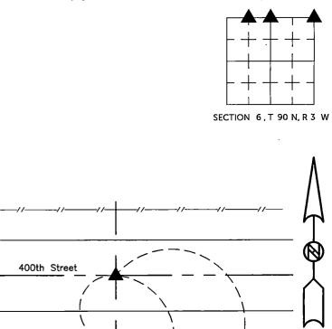
N 1/4 Corner Set 1/2"Ø Rebar with Orange Plastic Cap PLS 17939
