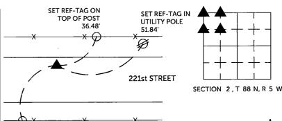
**NE CORNER NW 1/4 - NW 1/4** SET 1/2" REBAR W/ORANGE CAP #17939 8' NORTH OF CENTER LINE
