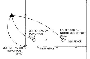
**SW CORNER NW 1/4 - NW 1/4** SET 1/2" REBAR W/ORANGE CAP #17939 3' WEST OF FENCE
