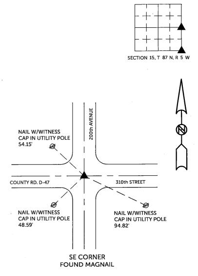
TIES ARE TO PLAT IN SECTION 15, T 87 N, R 5 W
